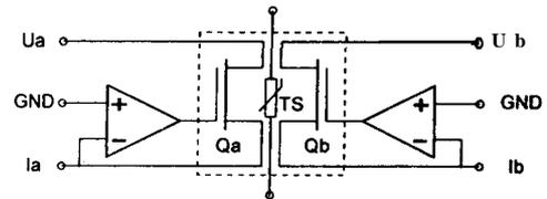
Fig. 2. Principal diagram of dual TTTC.
