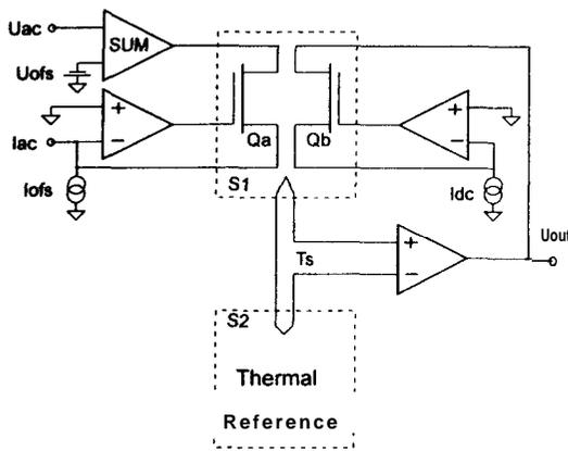
Fig. 3. Automatic self-balancing thermal bridge.
