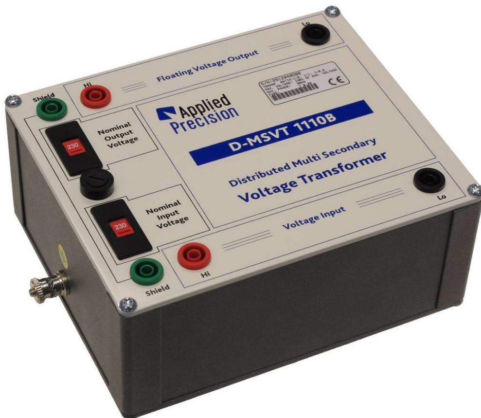
Basic Unit of the Distributed Multi Secondary Voltage Transformer D-MSVT™ system
