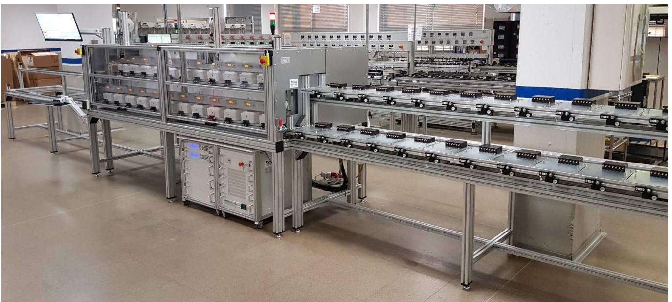
Electricity Meter Test Equipment ELMA with horizontal meter placing - fully automatic (customized, horizontal meter placement)
