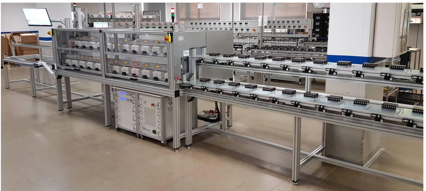
Electricity Meter Test Equipment ELMA with horizontal meter placing - fully automatic
