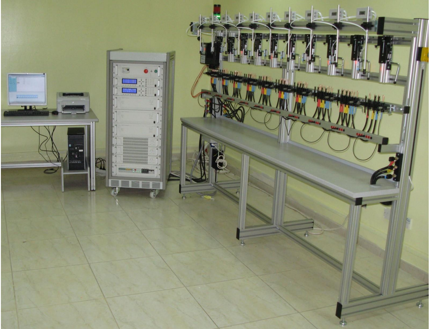
Electricity Meter Test Equipment ELMA with Fixed Meter Handling System
