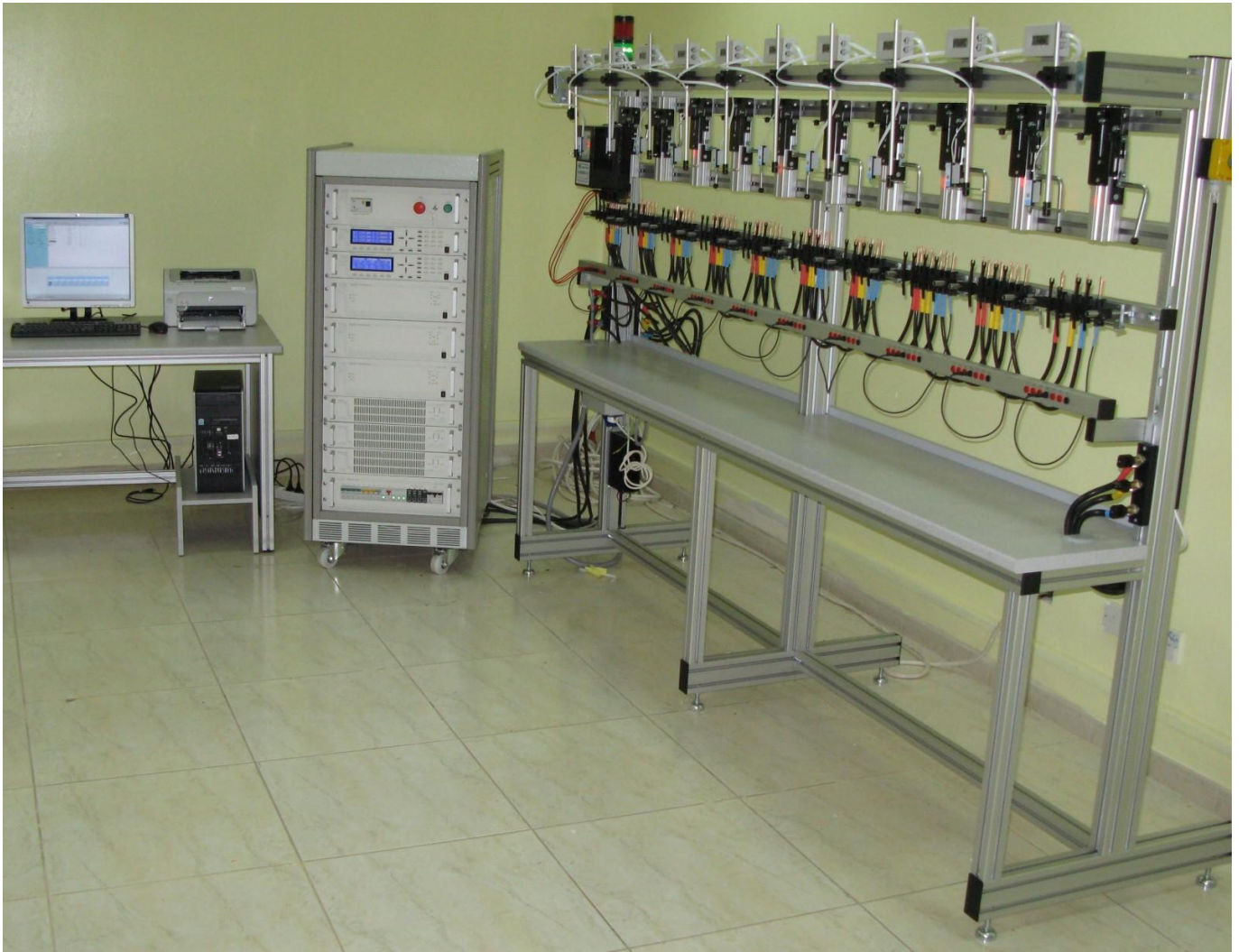
Electricity Meter Test Equipment ELMA with Fixed Meter Handling System (standard, vertical meter placement)
